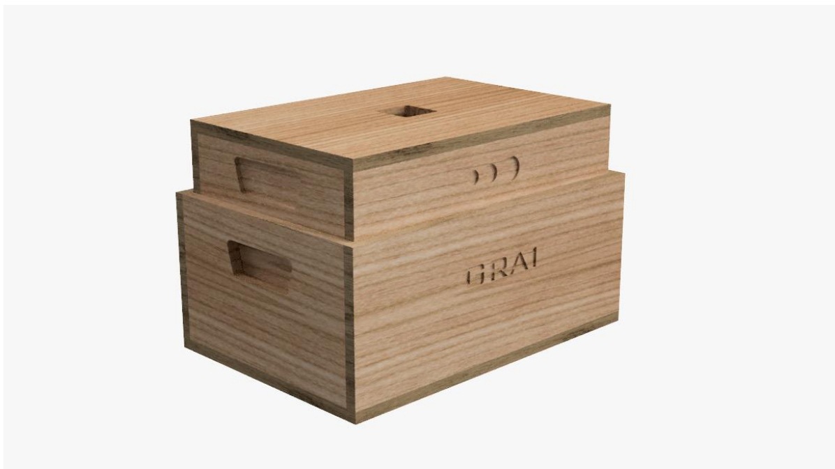
Figure 2. Rendering of the photo box for image acquisition.
